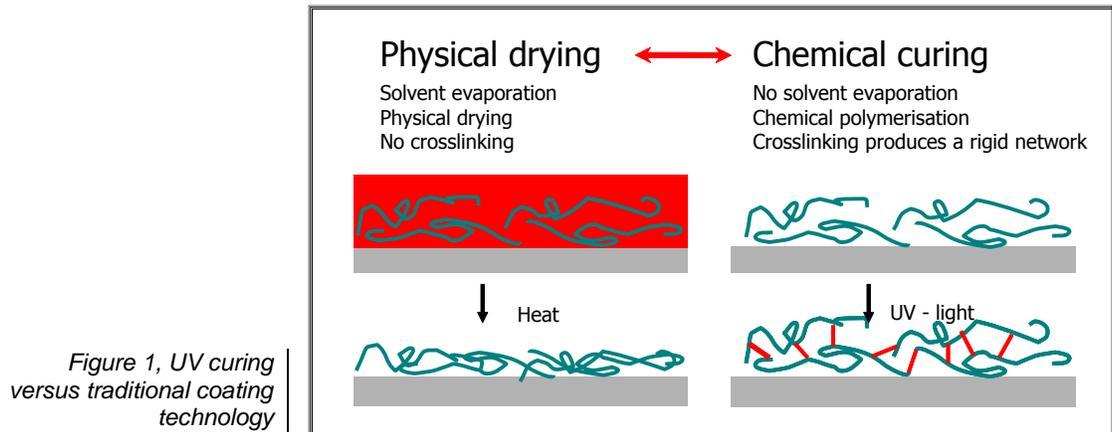
Figure 1, UV curing versus traditional coating technology
