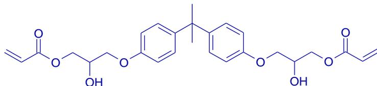
Figure 3, example of an epoxy acrylate
